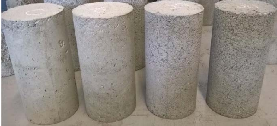
Hardened concrete blocks with various weight of vinyl flooring showing density (0 percent, 10 percent, 20 percent, 30 percent), Boral Lab 10
