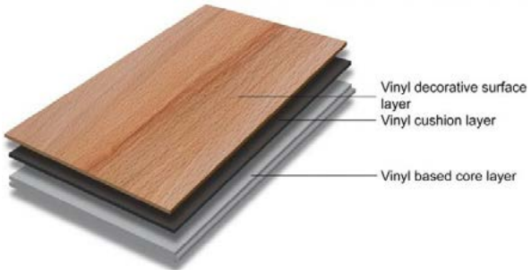
Figure 13: Examples of structure of LVT products
