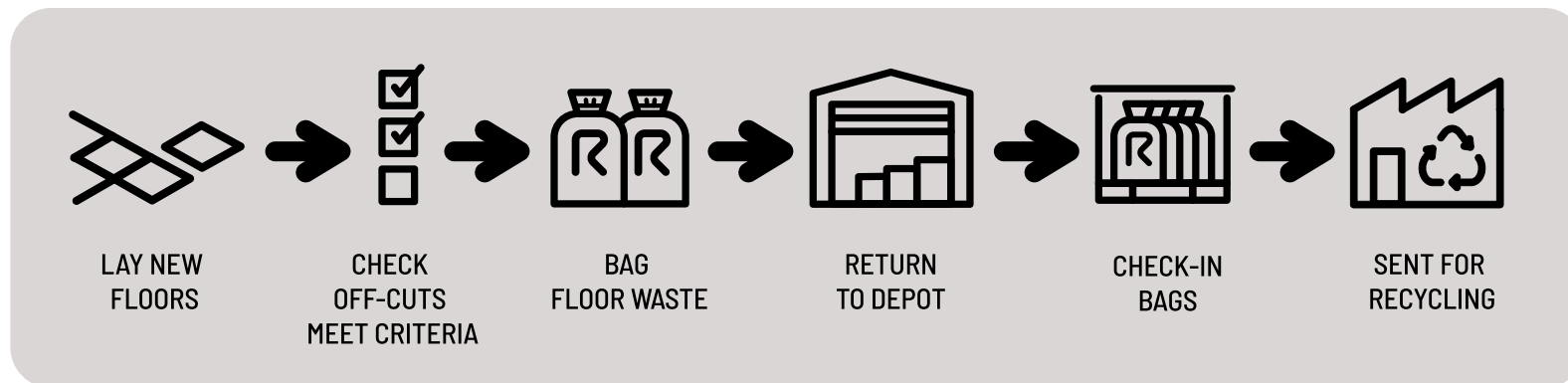
Figure 5: ResiLoop material recovery process
